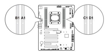
4 DIMMs working simultaneously
